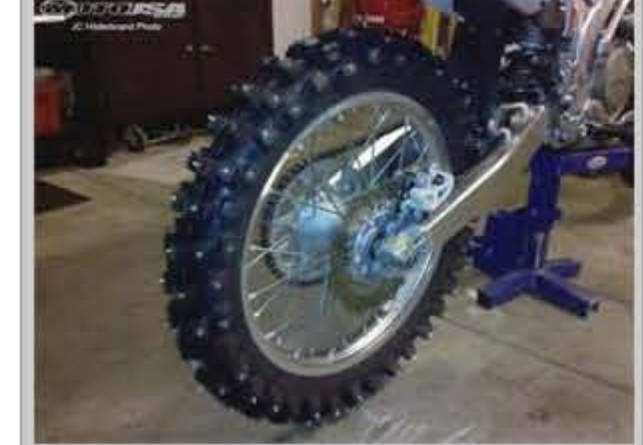
(Bottom) Tires like IRC, which are known for extra-deep lugs, are recommended. Notice the damage to the concrete floor simply from spinning wheel lightly during installation.
