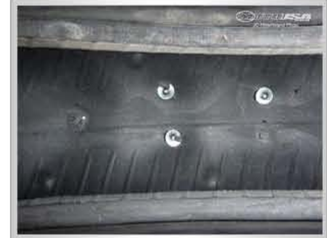
(Top) Using a worn-out tire results in this. We had to pull all the studs and start with a fresh tread.
